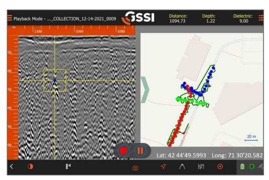
Data on the left side of the screen shows a typical utility at 1.25m in depth and shows a nicely defined base layer at .4m in depth. The blue dot on the data image is a water line.
