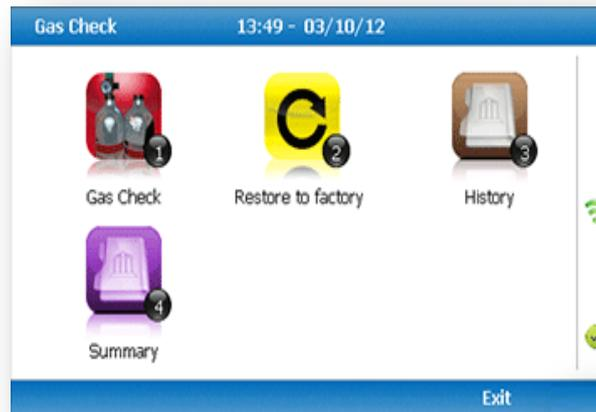
This option will reset the gas analyzer to all of its factory programmed calibration settings and will clear ALL the user defined calibration points. **It will not affect or remove ID's or readings from the analyzer.**
