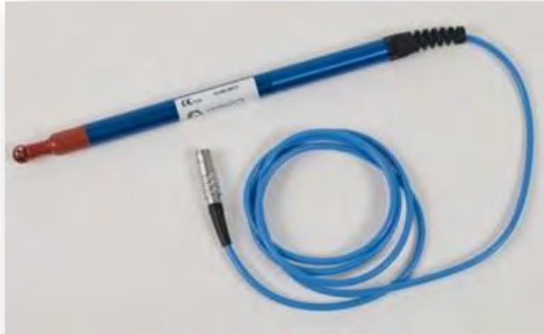
The GEM5000 gas analyzer has the facility to attach an anemometer device enabling the site engineer to measure the flow of gas within an extraction system. The anemometer can be set to display two values; m/s (meters per second) and m<sup>3</sup>/hr (metres cubed per hour).
