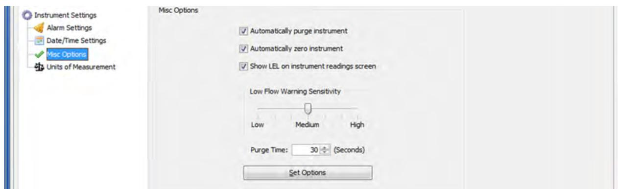
Under the miscellaneous options interface the user can change the following instrument settings:
